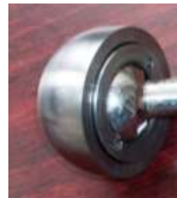
Figure 7. Acetabular cup - femoral head joint with balls in self directed movement (SDBJ).
